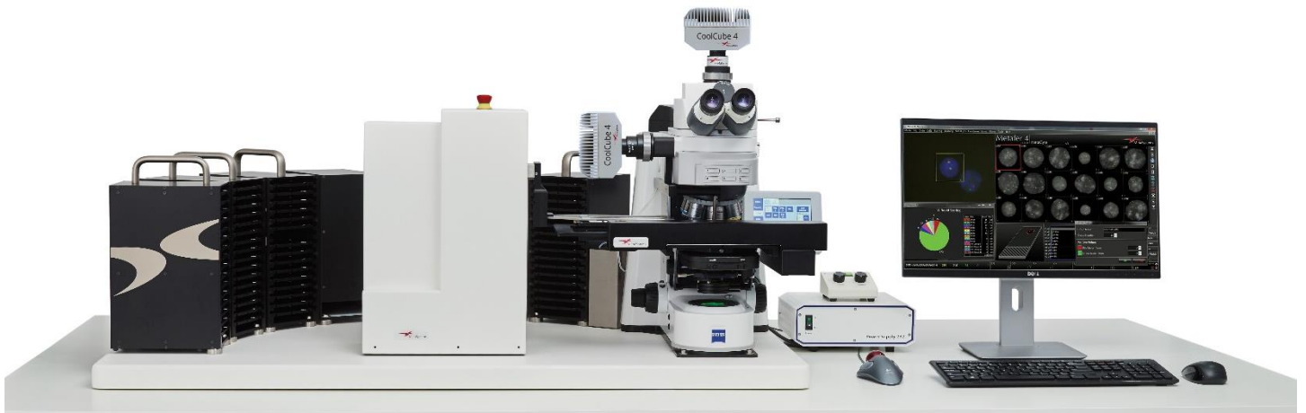
Figure 5: Metafer-driven slide scanning installation for interphase FISH spot imaging. This includes a motorized microscope fitted with one or two cameras, along with a stepping motor stage. To enhance scanning capabilities, an automated slide-feeding robotic device (SlideFeeder x80; positioned on the left) can supply up to 800 slides per run to the microscope stage. Additionally, a barcode reader is integrated to automate slide identification and allocate samples to respective cases and Search Information Files (SIFs).
