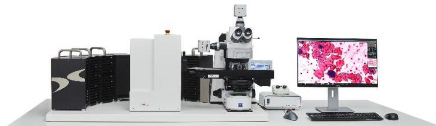
**Figure 1.** Gram Scanner instrumentation equipped with a Zeiss Axioimager Z2 microscope, CoolCube color camera, slide feeder, and magazines.
