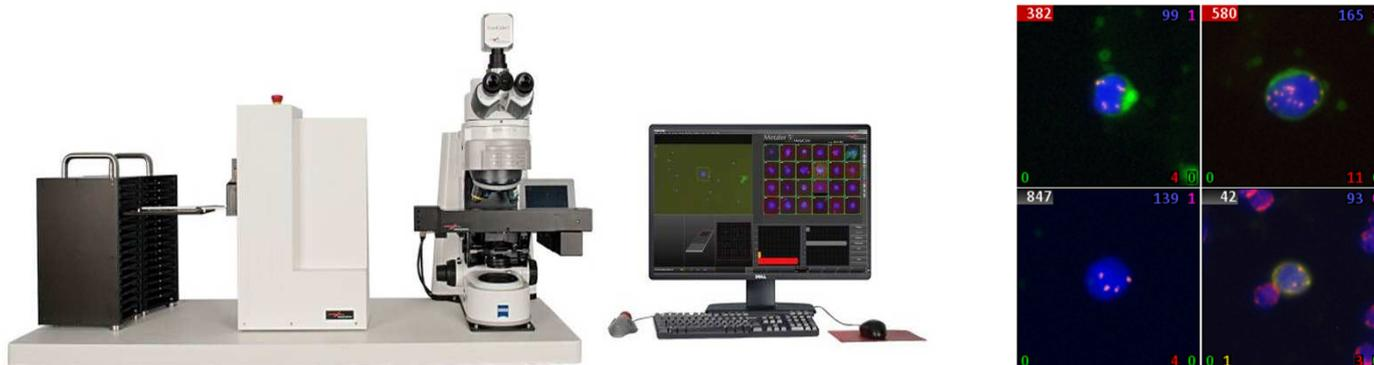
Figure 3: The Metafer CTC platform with full SlideFeederX robotic module, which increases capacity in modular 80-slide units. Example gallery of circulating endothelial cells (CECs) and both marker negative and positive CTCs identified by the Metafer CTC Application. CECs can be identified by CD31 staining (see Lin et al., 2017 for a comprehensive guide).
