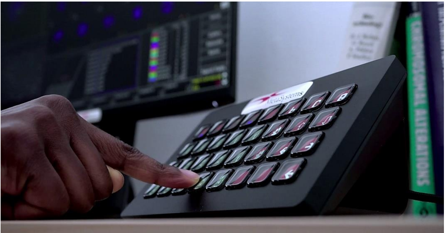
Figure 2: The programmable RapidScore keyboard allows instant confirmation or correction of automated outputs with just one keystroke.
